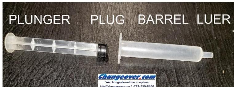
Syringes also have a plunger or rod, threaded or snapped into the plug. In use this pushes the plug down dispensing product through the luer. This is often inserted after filling and plugging are finished. In some cases it is not assembled to the plug but shipped with the syringe for assembly at point of use. This means one less operation for manufacturing to worry about.
