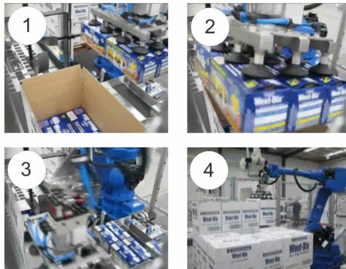
In a vertical placing system the product is must first be collated and isolated in a staging area. A 4 X 3 pattern for vertical pickoff can be collated by dividing the flow of products into 3 lanes, then using hold-backs to release backpressure on the last 4 products in each lane. The robot arm, with 12 grippers or suction cups, picks up the entire pattern and places it in the case
