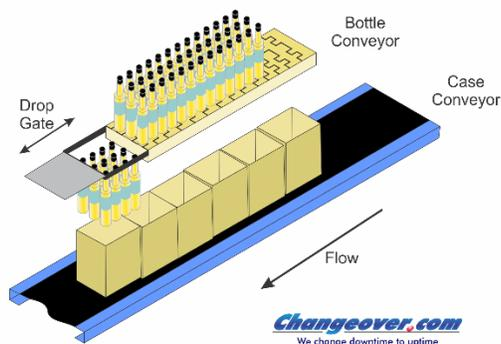
While the bottles are staging, an empty case is positioned under the staging area or drop grid. This case is often raised so as to minimize the vertical drop from staging to the case bottom. Some designs lower the case as the bottles drop reducing the shock. Once case and bottles are in position, the gate is opened and all products drop simultaneously into the case. Fingers between each bottle help guide them into position as they fall.
