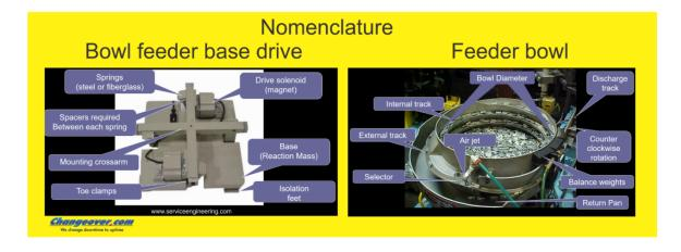
If the springs were mounted vertically, this back and forth movement would merely jiggle the product without causing motion. Instead, the springs are mounted on a slight angle opposite the direction of flow. As the magnet pulls the track back, the angle causes it the track to move down. As the magnet releases, the track moves up as it moves forward.
