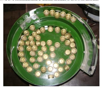
This photo shows an active selector. Parts are oriented lengthwise and passed by a camera. The camera detects incorrectly oriented parts and blows them back into the bowl.
