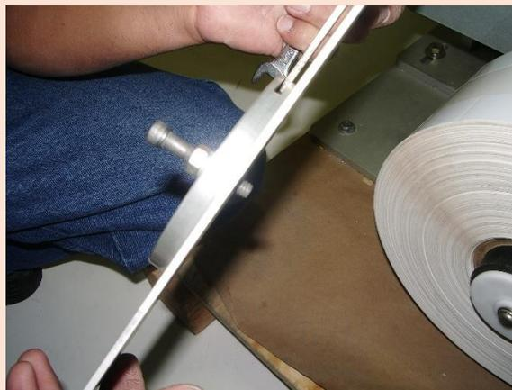
A disk on the axle, supports and positions the roll. On a vertically mounted head, as shown, a second disk or cross piece helps hold the roll in position.
