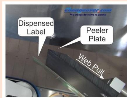
As the backing web bends, the label has a tendency to continue straight as it releases from the web. Some thinner materials or more aggressive adhesives may not want to release smoothly. One or more jets of compressed air (not shown here) directed at the label can aid release.
