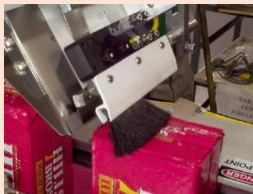
When using direct dispensing like this, synchronizing conveyor and labeler dispense speeds electronically is highly recommended. Depending on mechanics, and especially operators, to keep them synchronized manually is seldom reliable.
