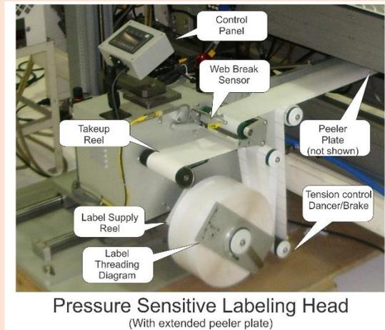
This picture shows a typical PS labeling head with the major components identified.
