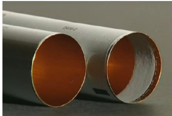
The flattened end of the tube is then folded in successive stations. Shown are a single and a double fold crimp. Other crimping configurations may sometimes be used.
