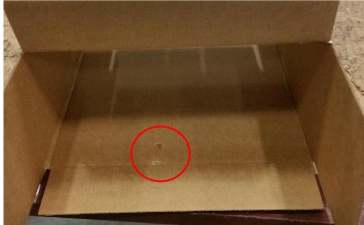
This picture shows a corrugated case but the glue problem is similar. Excess glue from the manufacturer’s joint has glued the knocked down case shut. This may prevent it from opening properly and causing a jam. Stronger opening grippers may rip it open but at the cost internal damage.
