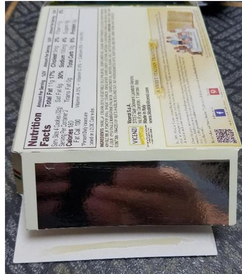
The carton on the right has an additional issue with the chrome coated major flap. Glue likes a rough surface to cling to. The chrome coating may not allow the glue to adhere properly even if everything else is right. Glue areas must always be unvarnished for best adhesion.
