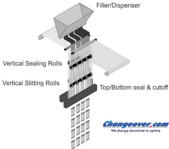
Schematic of continuous motion, 4 side pouch machine
