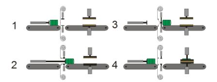
If higher speeds are required, some machines will have 2 pairs of rolls, side by side. This configuration operates the same as described above except that there are 2 bundles being wrapped on each cycle.
