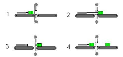
If a true a full 6-sided wrap is required, side sealing bars can be added after the initial 4-sided wrap. These are 2 pairs of sealing jaws, one on each end of the bundle. The bundle pauses at the jaws and they close, sealing the ends of the film together and, generally, cutting off any excess. When fully sealed in this way, a means for escape of trapped air must be provided to allow the film to shrink conformally and avoid the pillow effect mentioned earlier.
