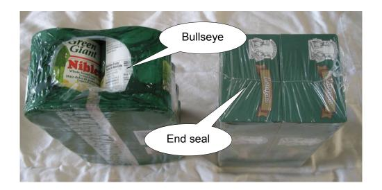
Many products in the past were packaged in corrugated trays prior to shrink wrapping. This adds considerable cost to the product as well as an additional production step and machine. Higher performance films have allowed the reduction and elimination of corrugated board. This picture shows beverage cans in a corrugated tray of 24 cans and in a trayless wrap of 28 cans.
